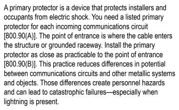
If you're installing phone cable, ground the metallic sheath (or interrupt it by an insulating joint) as close as practicable to the point of entrance [800.100]. This rule applies to other types of cable covered by Articles 810, 820, and 830.
